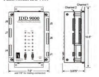
The PM IDD 9000 is available as single or dual channel. The dual channel has a separate, identical PCB motherboard for each channel. Each board contains six connectors on the side panels. Dual channel shown, bottom board is removed on single channel configuration.
