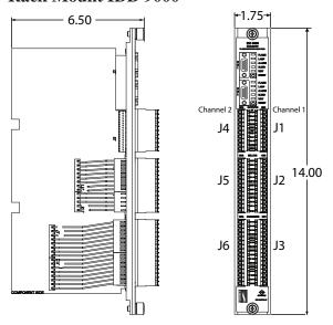
The RM IDD 9000 is a dual channel amplifier with a separate identical CPU Processor for each channel. The right side is for Channel 1 and the left side is Channel 2. The RM IDD 9000 is designed for installation into an amplifier rack (Part # 404325-02) in an equipment cabinet.
